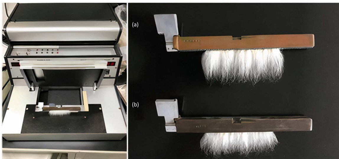
Figure 1. Fiber Strength measurement (a) Long strong with 30.5 mm and (b) Short-weak with 19.2 mm.
