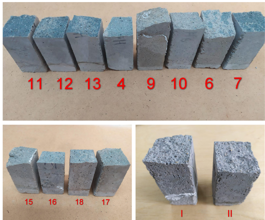
Figure 10. Appearance of samples after the efflorescence test.
