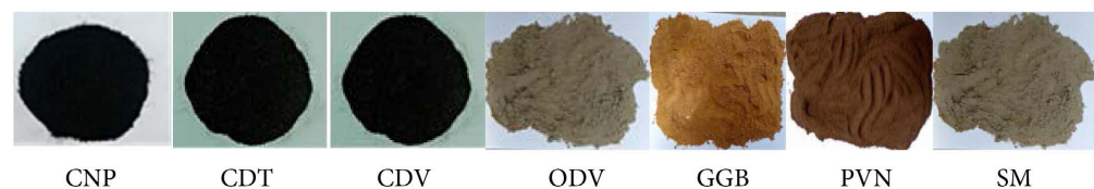
Figure 1. Testing samples. Note: CDT: Bull horns, CDV: Cow horns, ODV: Cow bones, CNP: Oil palm nut shells, SM: Mwenga salt, GGB: Ginger t, PVN: Black pepper.
