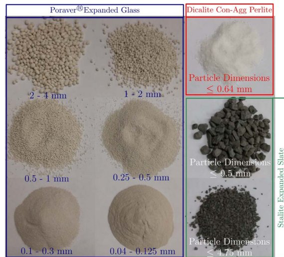
Figure 1. Particle sizes of three light-weight aggregate types.
