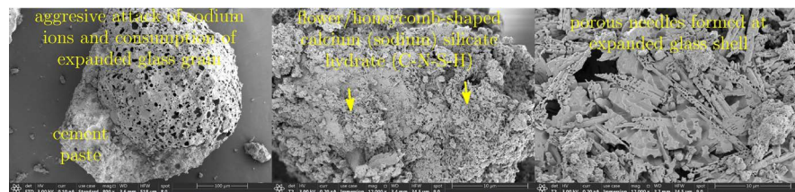
Figure 13. SEM images of 26-hour mortar with expanded glass as aggregate and 20M NaOH aqueous solution mixed with cement as the binder (sample U1 in Table 3 ) exposed to ultra-accelerated ASR regime.
