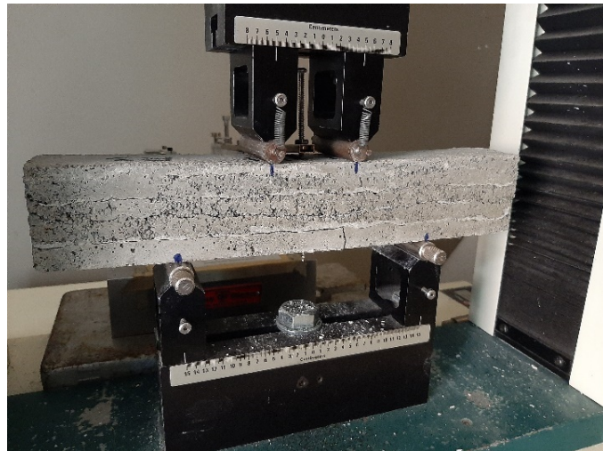
Figure 13. Failure pattern of L-nF samples.
