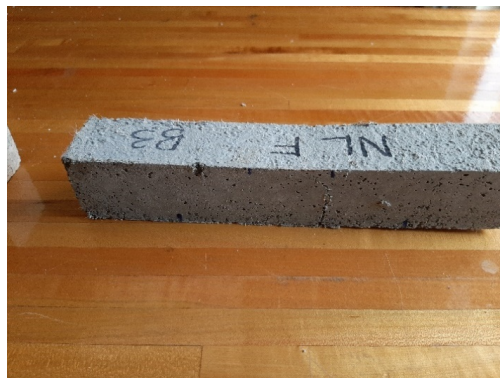
Figure 10. Failure pattern of nL-F samples.
