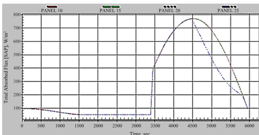
Figure 6. Total absorbed fluxes w.r.to time for all nodes on the panel in shooting mode.
