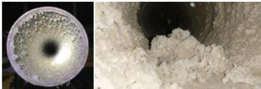
Figure 10. A significant buildup problem with resin pellets in a conveying line due to a leak.
