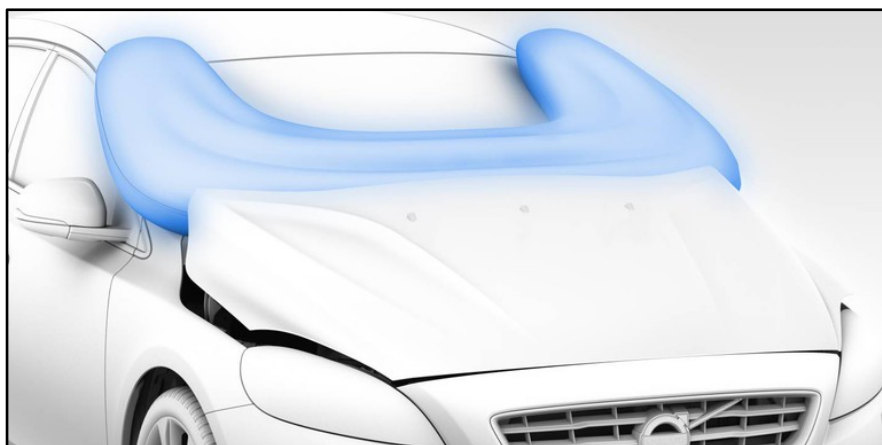
Figure 6. Artist's impression of Volvo's pedestrian airbags.
