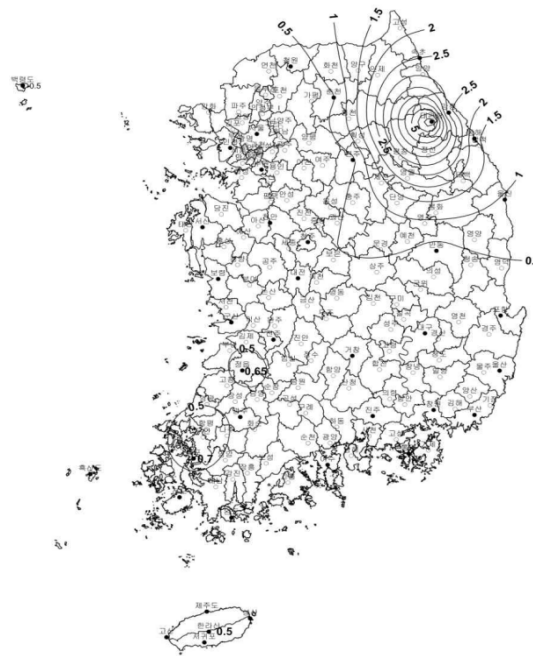
Figure 4. Design of the snow load (KBC 2016).
