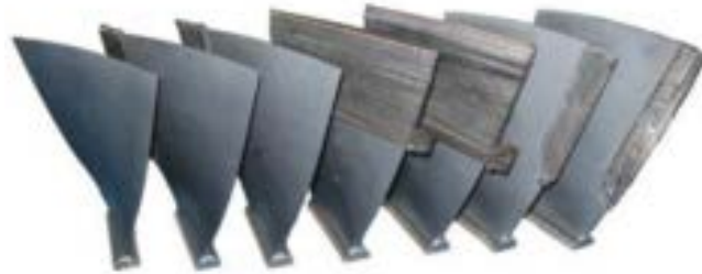
Figure 6. The repaired turbines via AM.
