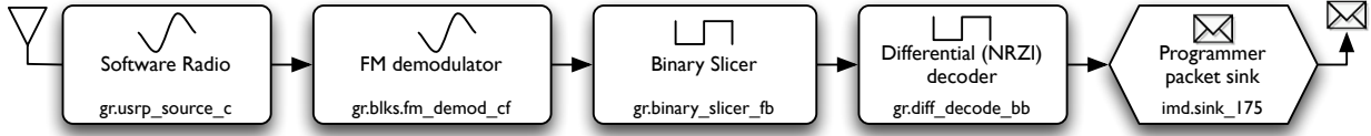
Fig. 6. Architecture of a GNU Radio-based eavesdropper. The purpose and Python class name of each signal processing block is included, as well as the format of the data it processes. All blocks but the last are from GNU Radio’s built-in block library. We adapted the last block, our imd.sink_175 packet framer, from built-in GNU Radio blocks.
