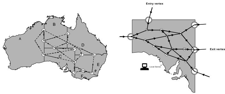
Figure 1. The global virtual graph (left) and a local traffic graph of region C (right)
