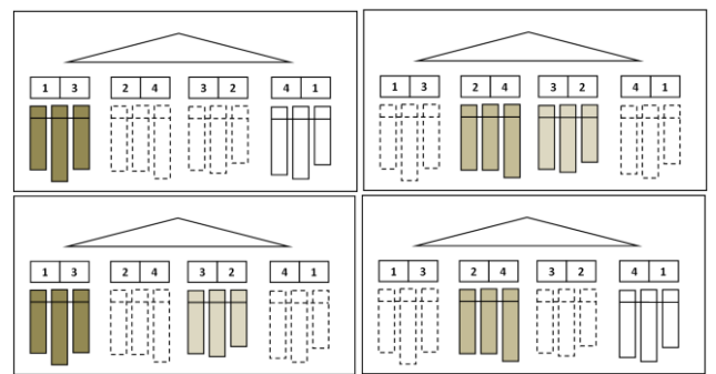
Figure 12. Logical view of in-memory home location index on completion of 1-safe distribution across 4 RAC instances.
