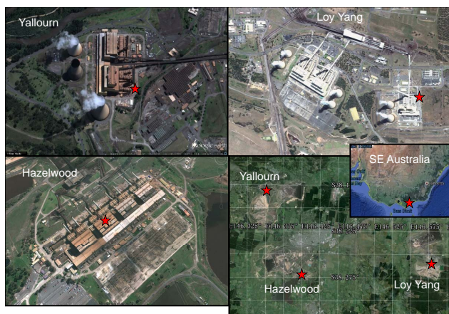
Fig. 7. The locations and aerial photos of the three coal power plants in the La Trobe Valley, Australia. The stars mark the base of the chimneys in the three zoomed-in photos. The power generation capacity is 1450 MW for Yallourn, 1600 MW for Hazelwood, and 3250 MW for Loy Yang.
