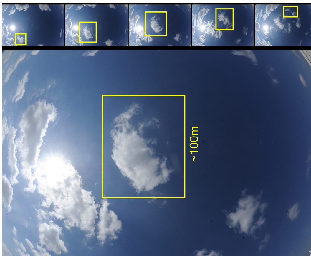
Figure 1. Images taken during a field campaign on 30 June 2011 at 15:52–15:56 LT. Top: sequential (1 min time lag) images of the complete lifetime of a single short-lived cloud. The camera was pointed at the zenith and the diagonal field of view is 180°. The yellow rectangles mark the position of the cloud. Bottom: enlargement of one of the images.
