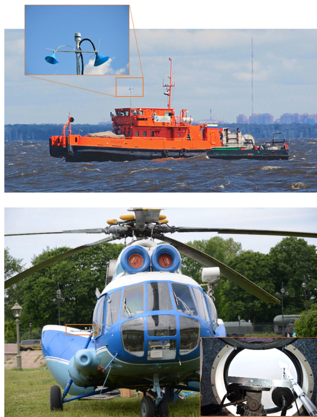
Figure 3. Top: work vessel Redut with sample inlets (photo of Redut taken by M. Pingoud); bottom: Mi-8 helicopter with sample inlet.
