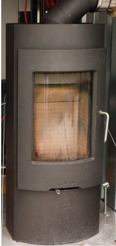
Figure S1. Photograph of residential wood burner used for all burning. The stove is not fitted with a catalyst or other emission control device.
