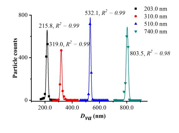
Figure S1. Gaussian fitting for the  $D_{va}$  size distribution of an aerosol of spherical PSL particles with  $D_{ve}$  values of 203.0 nm, 310.0 nm, 510.0 nm, and 740.0 nm after screening by the AAC.
