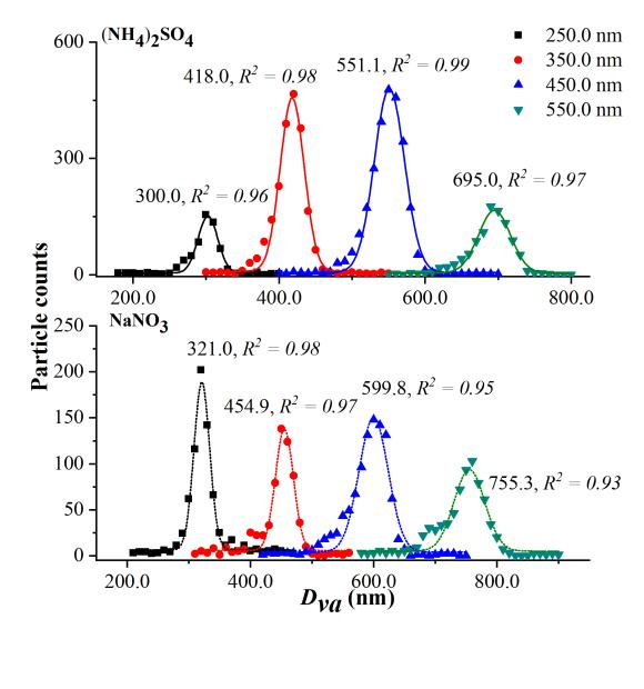
**Figure S2.** Gaussian fitting for the  $D_{va}$  size distribution of the aspherical aerosol particles of (NH<sub>4</sub>)<sub>2</sub>SO<sub>4</sub> and NaNO<sub>3</sub> with  $D_a$  values of 250.0 nm, 350.0 nm, 450.0 nm, and 550.0 nm.
