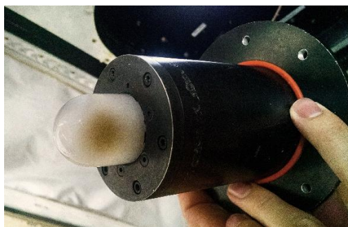
262 Figure S13. Strong aerosol contamination of the optic following the flight on 19 May, 2016.
