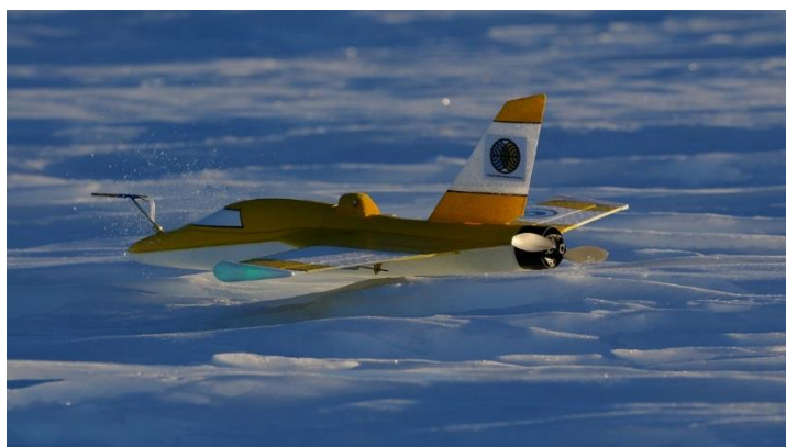
Figure A1. Small Unmanned Meteorological Observer (SUMO), which is used to measure vertical profiles of air temperature, humidity and wind speed up to the height of 2-3 km. Photo Priit Tisler, Finnish Meteorological Institute.
