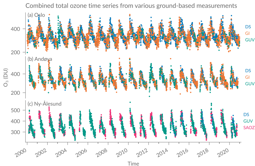
Figure 2. Daily means of total ozone from four different measurement techniques: Brewer Direct Sun (DS), Brewer Global Irradiance (GI), ground-based UV (GUV), and SAOZ, measured at (a) Oslo, (b) Andøya, and (c) Ny-Ålesund. DS data are the main dataset in Oslo (a) and Andøya (b), days without DS measurements are filled with GI data, remaining missing data are then filled with GUV measurements. In Ny-Ålesund (c), SAOZ is the main dataset, and DS and GUV are used to fill days with missing SAOZ data.
