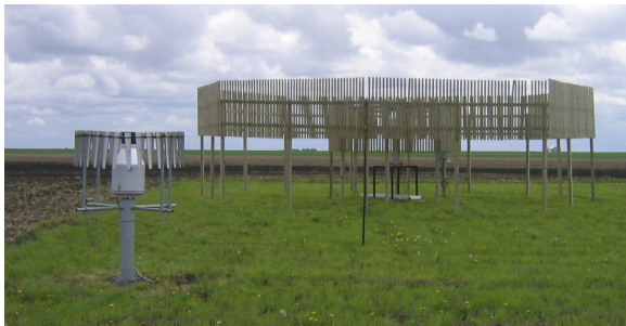
Figure 2: Alter-shielded Geonor T-200B (left) and a Geonor T-200B in a large octagonal double fence (right).
