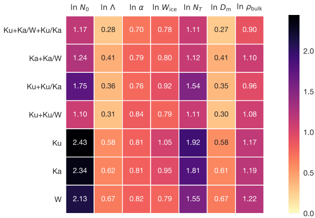
Figure 5. The average posterior retrieval errors of the logarithms of microphysical variables with different combinations of radar frequencies. The data from the 4 December 2015 case (Sect. 5.2) are used in this figure.
