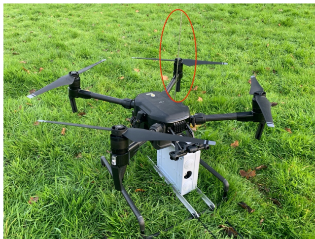
Figure 1. The DJI Matrice 200 V2 with the POPS (white box at the left bottom of the fuselage). The red oval shows the inlet tube leading to the POPS.
