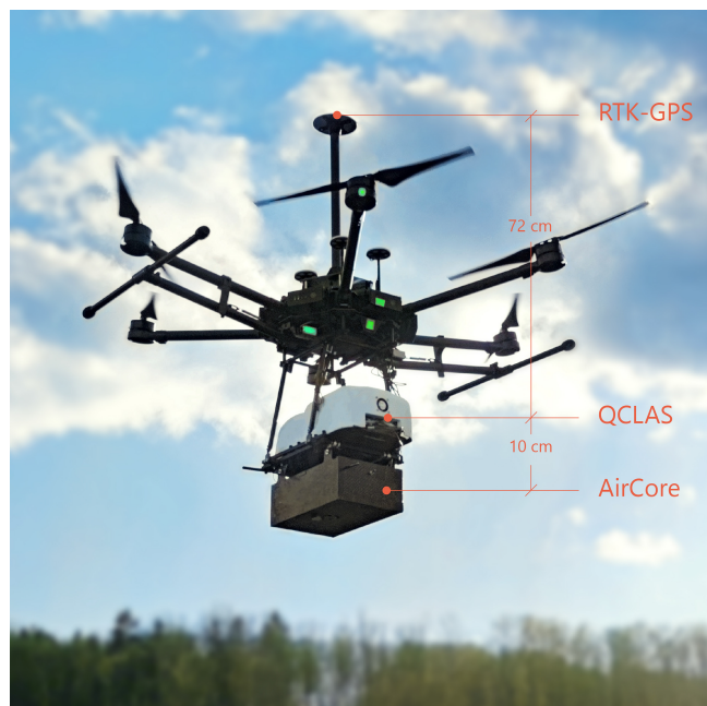
Figure 1. The embedded UAV system used for CH 4 detection: the QCLAS analyser and the active AirCore sampling system are mounted below a Matrice 600 DJI hexacopter equipped with an RTK-GPS system.
