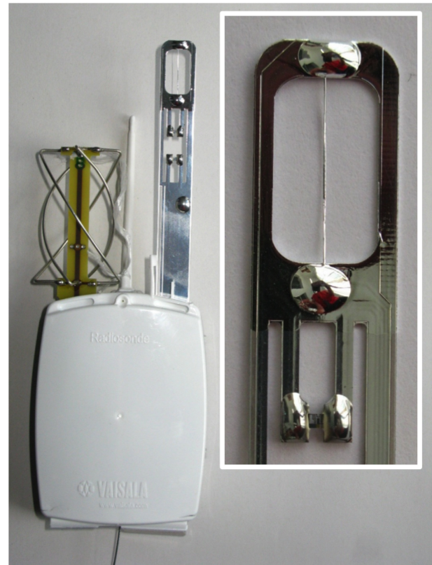
Figure 1. Photograph of the RS92 radiosonde showing the GPS antenna on the left and the sensor boom on the right. The inset shows the magnified tip of the sensor boom with the wire-shaped temperature sensor and one of the humidity sensors.
