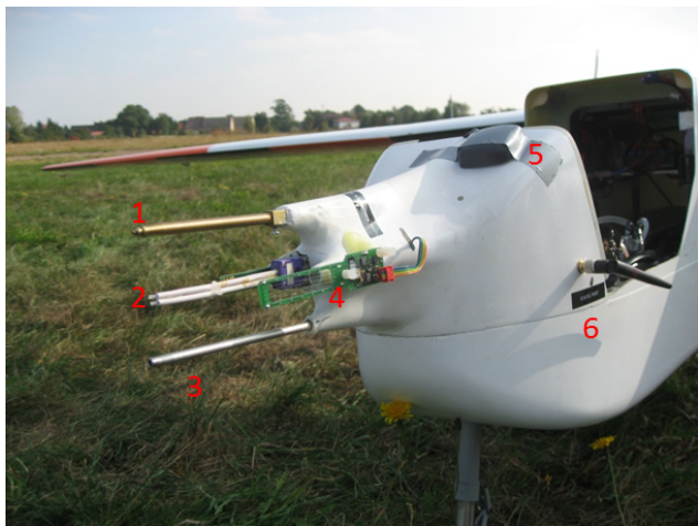
Figure 2. The meteorological payload is mounted at the tip of the aircraft. The components are (1) five-hole probe, (2) temperature sensor (thermocouple) and humidity sensor P14 Rapid, (3) aerosol inlet, (4) fine wire platinum resistance thermometer, (5) GPS antenna and (6) telemetry antenna for real-time data transfer.
