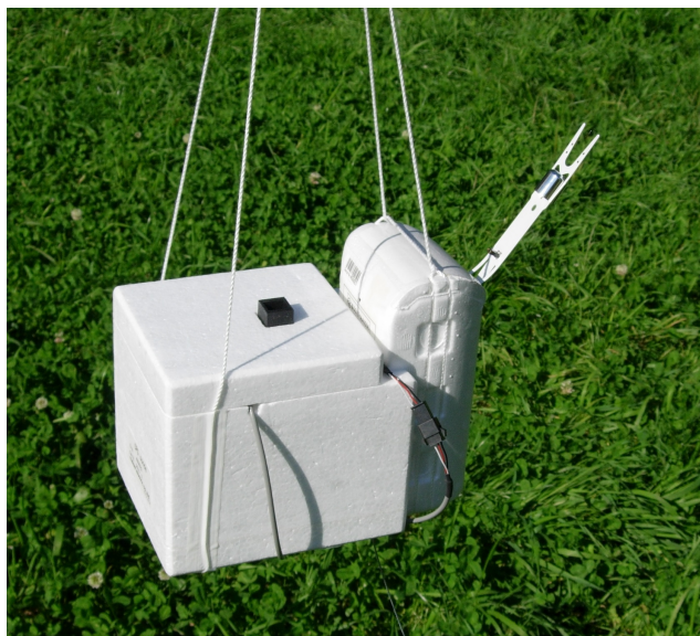
Figure 2. Photograph of the latest version CPS within its flight package (with a black inlet duct on top) connected to the Meisei RS-11G radiosonde (with the temperature and RH sensor boom). The three 3-V lithium batteries and the interface board are placed within the CPS flight package.
