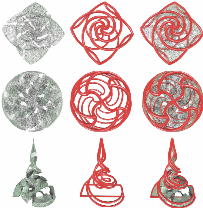
Fig. 8. Curve networks extracted from point clouds of objects with free-form surfaces.
