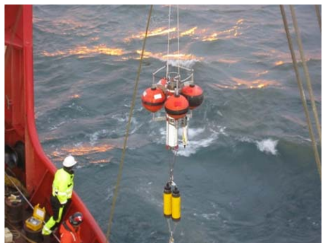
Fig. 5. Deployment of the IPSSL mooring in the Canadian Beaufort Sea, Sept. 2014 from the CCGS Sir Wilfrid Laurier vessel.
