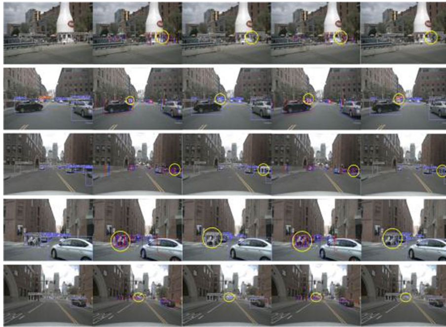
Fig. 7 Experimental effect of error detection compared with the baseline model is plotted. The first column is the estimated depth value on the image, which can visualize the specific target on the image and facilitate the experimental comparison effect demonstration; the second column is the 3D block diagram of the target detected by the baseline model; the third column is the specific classification and detection effect diagram of the target detected by the baseline model, which can directly reflect the target detection effect; the fourth column is the 3D block diagram of the target of our proposed CenterTransFuser model; the fifth column is the specific target classification and detection effect diagram obtained by our model
