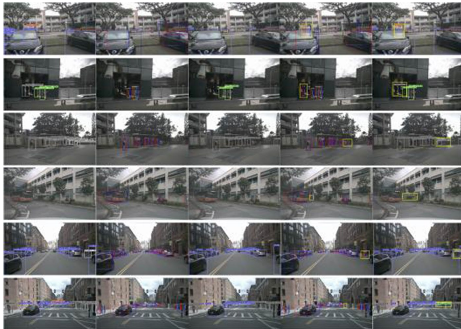
Fig. 6 Experimental effect of missed detection compared with the baseline model is plotted. The first column is the estimated depth value on the image, which can visualize the specific target on the image and facilitate the experimental comparison effect demonstration; the second column is the 3D block diagram of the target detected by the baseline model; the third column is the specific classification and detection effect diagram of the target detected by the baseline model, which can directly reflect the target detection effect; the fourth column is the 3D block diagram of the target of our proposed CenterTransFuser model; the fifth column is the specific target classification and detection effect diagram obtained by our model
