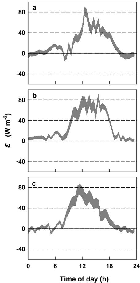
**Fig. 1.** Uncertainties in energy balance closure residuals ( $\varepsilon$ ) due to spatial variability in  $R_n$ . The upper and lower bounds of the gray band derived from the maximum and minimum  $R_n$  of the eight treatments, respectively. Site I, a, II, b, III, c. Data are derived from Experiment 1.
