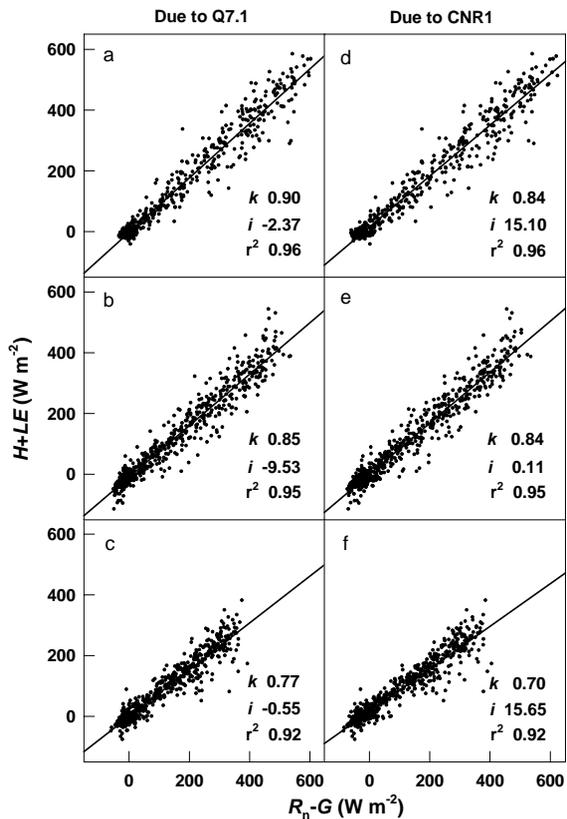
**Fig. 3.** Comparisons of 30 min values of turbulent ( $H + LE$ ) vs. available energy ( $R_n - G$ ) derived from Q7.1 “(Left)” and CNR1 “(Right)” determined  $R_n$  with the ordinary least square (OLS) linear regression equation of  $(H + LE) = k(R_n - G) + i$  ( $k$ , slope,  $i$  intercept, coefficient of determination,  $r^2$  are also shown). The solid line shows OLS linear regression fit. Site I, “a, d”; II, “b, e”; III, “c, f”. Data are derived from Experiment 1.
