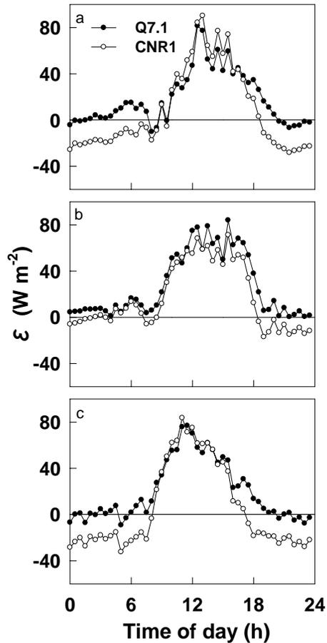
**Fig. 2.** Energy balance closure residuals ( $\varepsilon$ ) derived from Q7.1 and CNR1 measurements in  $R_n$ . Site I, a, II, b, III, c. Data are derived from Experiment 1. 30 min averages data from 12, 16 and 17 days at sites I, II and III, respectively, were compiled into one-day scale, the same as Fig. 1.
