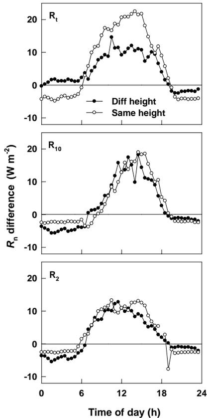
**Fig. 6.** Net radiometer deployment heights vs.  $R_n$  results (half-hourly data integrated into a diurnal scale). Diff height means  $R_n$  differences between the two Q7.1s deployed above the canopy by 0.5 and 1.5 m, respectively. Same height means both of the two Q7.1s deployed above the canopy by 0.5 m.  $R_t$ ,  $R_{10}$  and  $R_2$  see Fig. 5. Data are derived from Experiment 4.
