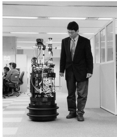
Figure 1: Jijo-2 robot is talking with a human user while it is navigating in an office corridor.
