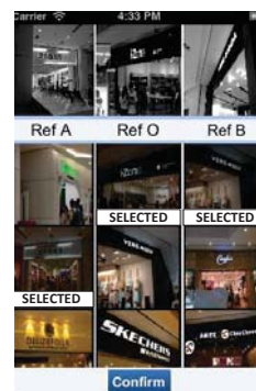
Fig. 17. The UI presented to the user for correction of image matching results. The top row are the 3 test images taken by the user, below each are the top 3 matched reference points. The user can denote the correct match by tapping the thumbnail images.
