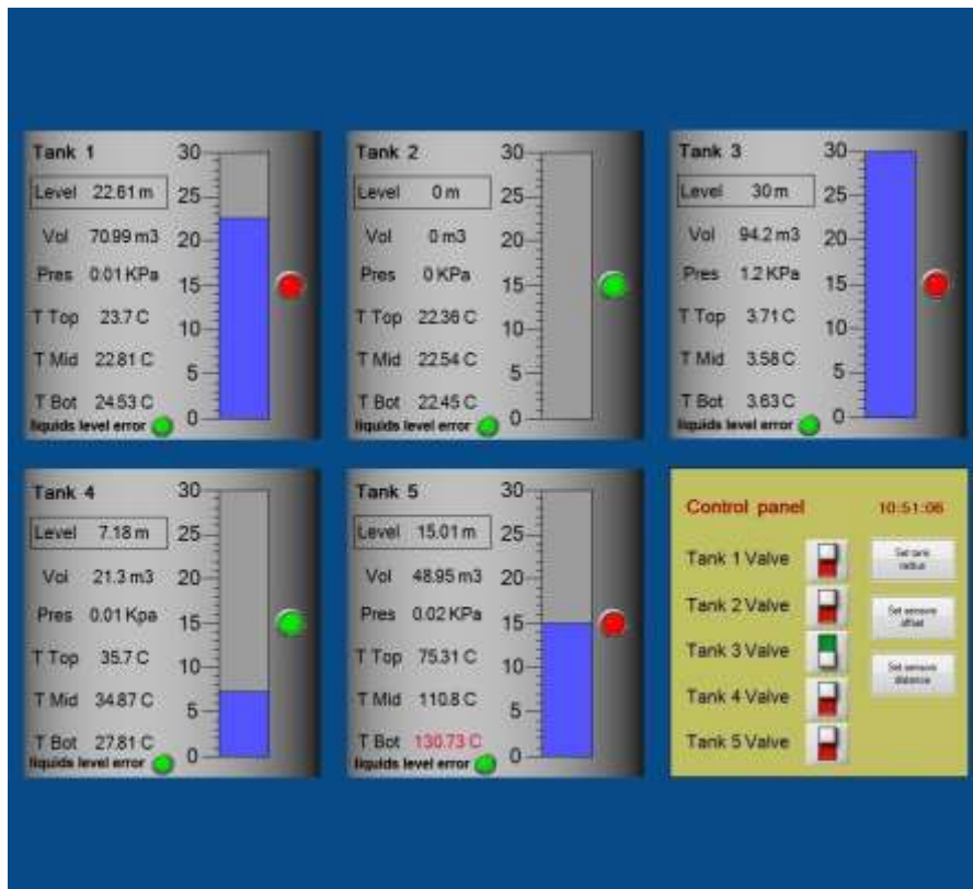
Fig. 3. Main screen of the HMI of the remote level control system with discrete self-testing.
