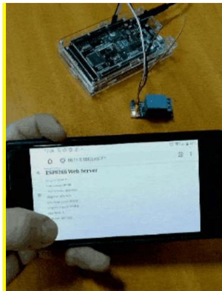
Figure 7: Wireless debugging of the control system
