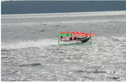
Figure 1: YOLO5 Small for the detection and tracking of a moving motorboat and people
