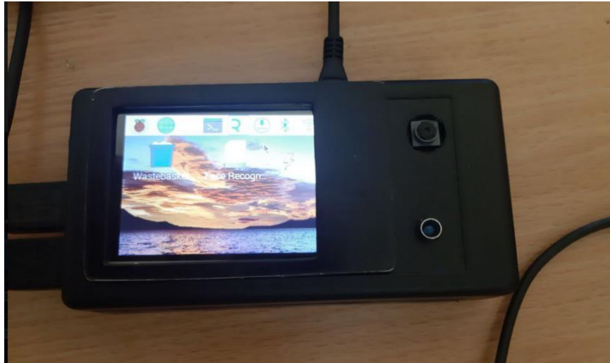
Figure 5. Laboratory stand for teaching students how to work with machine vision and face recognition
