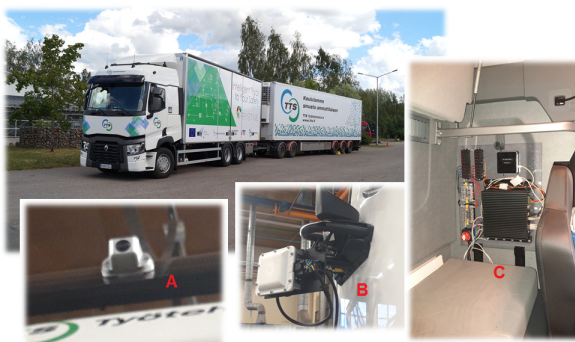
Fig. 24: Sensors mounted on the TTS heavy duty vehicle. A: front camera, B: side Radars, C: electronic equipment (cabin).
