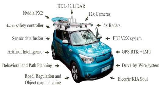
Fig. 7: EDI DbW car and its main components.
