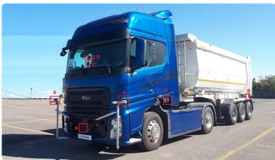
Fig. 20: Sensors mounted on the Ford heavy duty vehicle. A:Lidars, B: Radars, C:Smart-Camera, D:Stereo-Camera.
