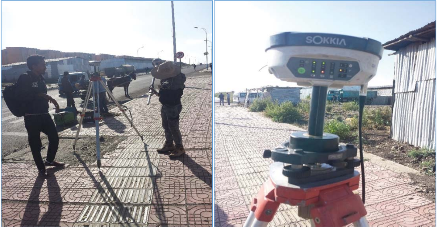
Fig. 2.4. RTK-DGPS adjustment at the base station (left) and the adjusted base station Receiver) (right)
