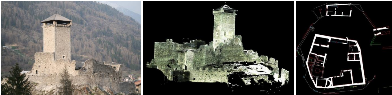
Figure 11. Range-based surveying of a medieval castle with TOF terrestrial laser scanning for detailed map production.
