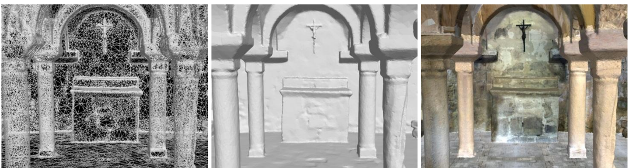
Figure 12. Different renderings (wireframe, shaded and textured mode) of a surveyed and modeled underground church.
