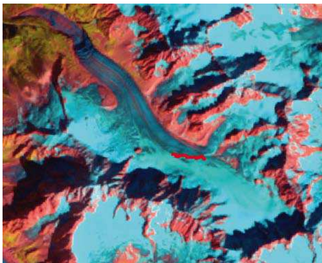
Fig. 2. Example of Landsat image used to delineate the snow line (red line) with a combination of spectral bands: green, near-infrared and shortwave infrared. Argentière Glacier (Mont Blanc Massif), Landsat TM5 image acquired on 9 September 1987.
