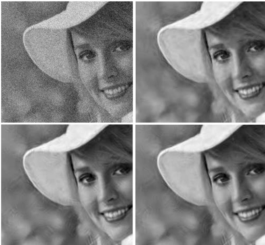
Fig. 11. Close-up of images. From top left, clockwise: Noisy image (PSNR = 22.12 dB), BivShrink DDWT (PSNR = 31.09 dB), NSST 1 (16, 32) (PSNR = 31.20 dB), and NSCT (PSNR = 31.15 dB).
