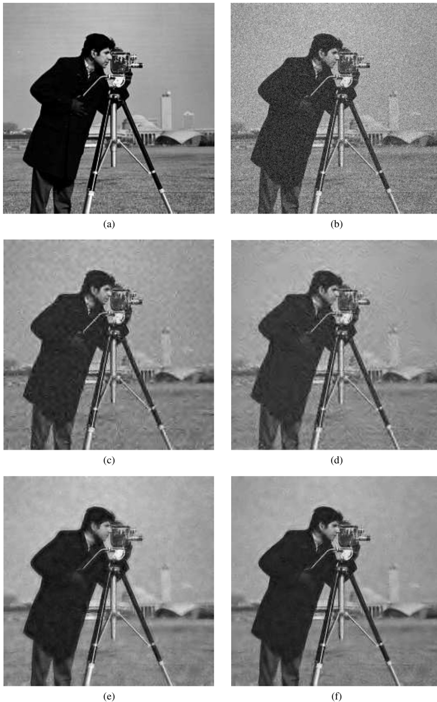
Fig. 9. (a) The original cameraman image. (b) The noisy image (PSNR = 22.09 dB). (c) The result of wavelet denoising using the 7/9 filters (PSNR = 26.18 dB). (d) The result of contourlet denoising (PSNR = 25.82 dB). (e) The result of the frequency-based shearlet denoising (PSNR = 27.21 dB). (f) The result of the time-domain shearlet denoising (PSNR = 28.01 dB).
