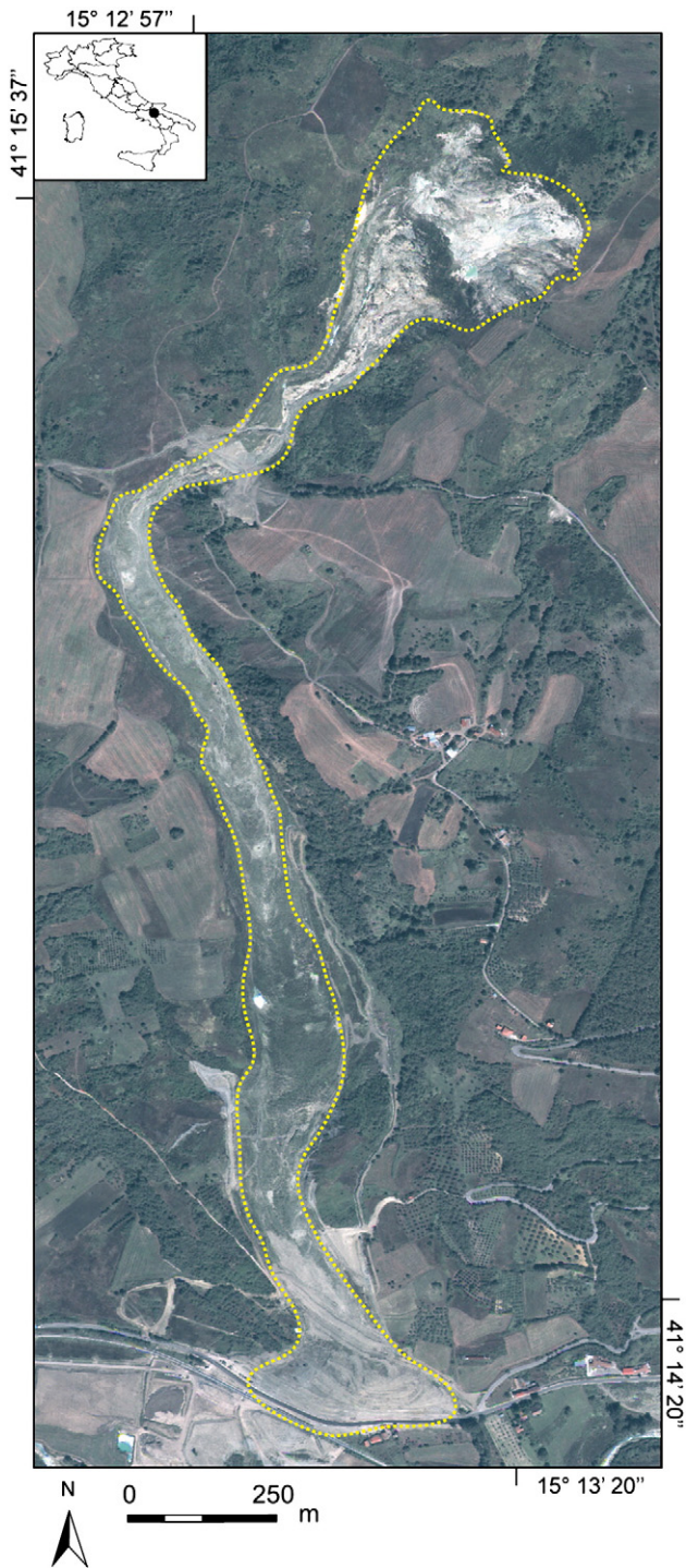
Fig. 8. Montaguto, Benevento, Italy, earthflow extending for 6.6 \times 10^5 \text{ m}^2 with an estimated total volume of 2.5 \times 10^6 \text{ m}^3 . Image captured by the GeoEye satellite on 20 October 2010. The yellow dotted line shows the boundary of the landslide at the date of the satellite image.
