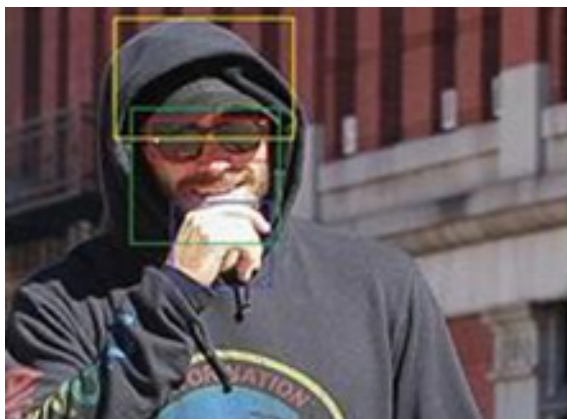
Figure 2: Detection of partially occluded faces, by considering sunglasses, caps and hands.
