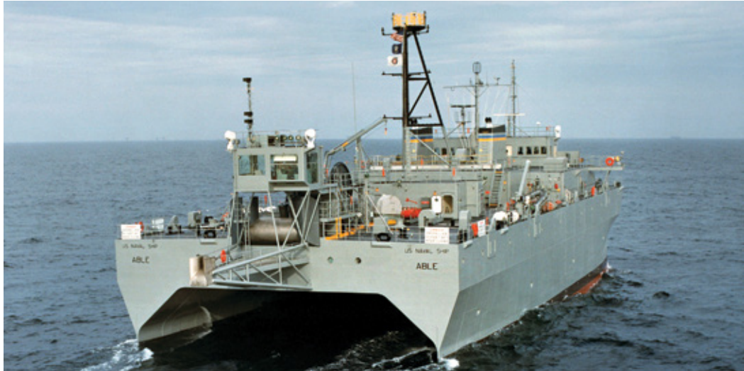
FIGURE 7: T-AGOS COMPACT LOW FREQUENCY ACTIVE SONAR SHIP
