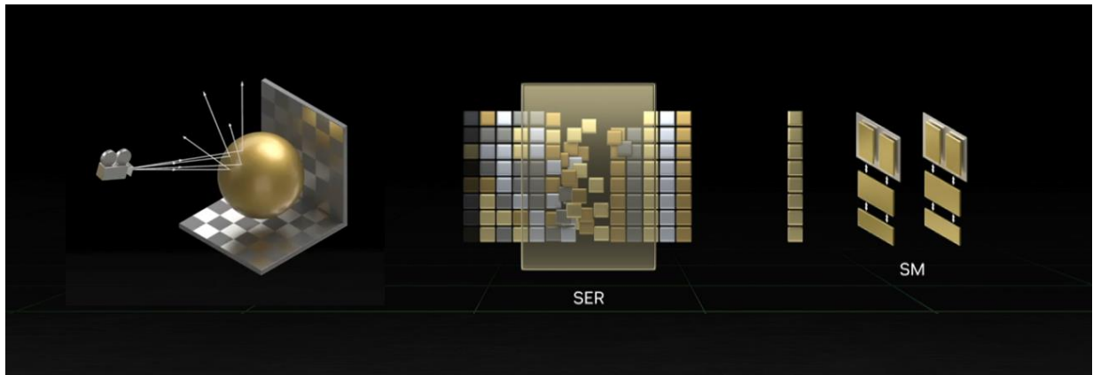
Figure 1: Left: rays bounce off an object in different directions, hitting different materials. Center: SER reorders threads, grouping similar work together. Right: SMs execute shaders with increased coherence.
