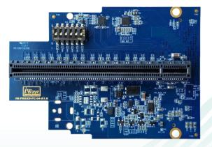
iWave's Gen4 x16 PCIe FMC+ Module is designed to meet VITA 57.4 FMC+ standard.
