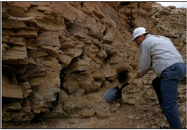
Figure 2A. A photo from right abutment site exploration in the 1950's showing the fractured nature of the foundation.
