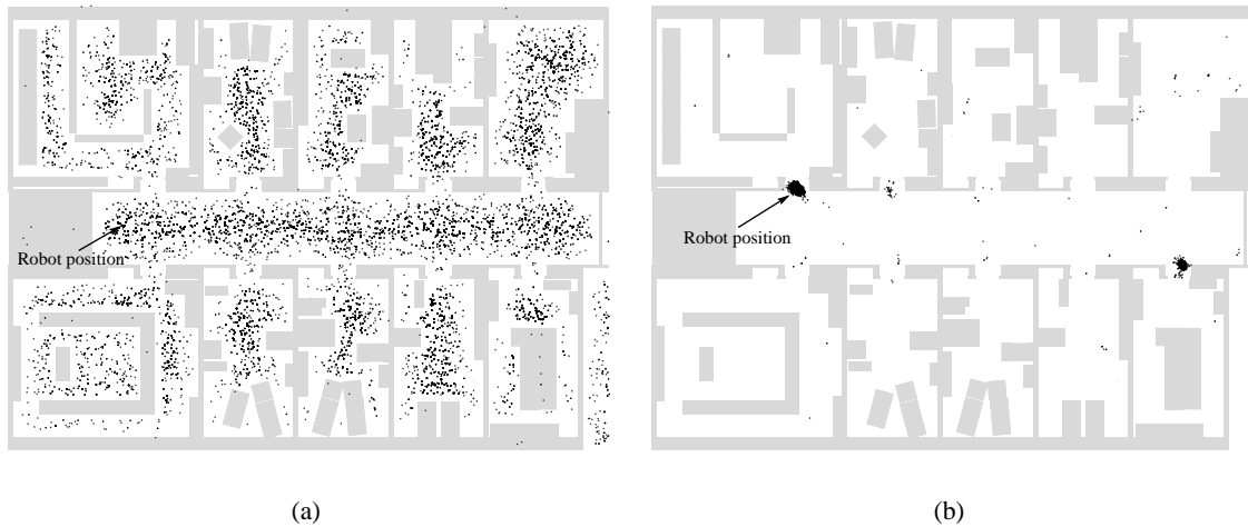
Figure 1: Monte Carlo localization of a mobile robot: the posterior density over the three-dimensional robot pose ( x , y , and orientation) is represented by a set of weighted particles which is sequentially updated over time (a particle filter). (a) Initially, the position of the robot is totally unknown, and particles are distributed uniformly over the environment. (b) After a number of sonar and odometry measurements, the uncertainty is reduced to essentially a bimodal density in this symmetric environment.
